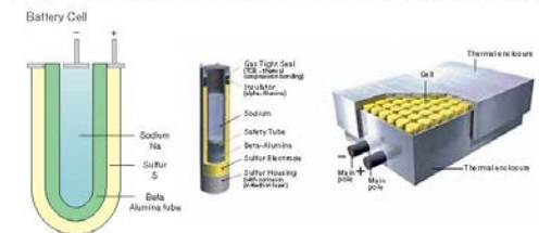
Figure 2-6 | NaS Battery: Cell design and 60 kW module (NGK, IEC MSB/EES Workshop 2011)
